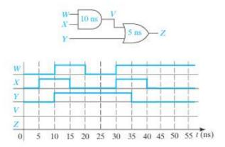
8.12 Complete the timing diagram for the given circuit. Assume that both gates have a propagation delay of 5 ns.
