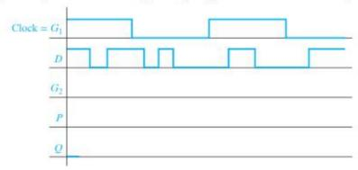
**11.11** Complete the following timing diagram for an S-R latch. Assume Q begins at 1.
